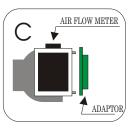
Fix the GREEN filter onto the air flow meter then fix it onto the air box support with the attaching bracket and the screw provided.(see diagram D)
