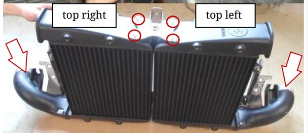
Dichtring / rubber sealing
