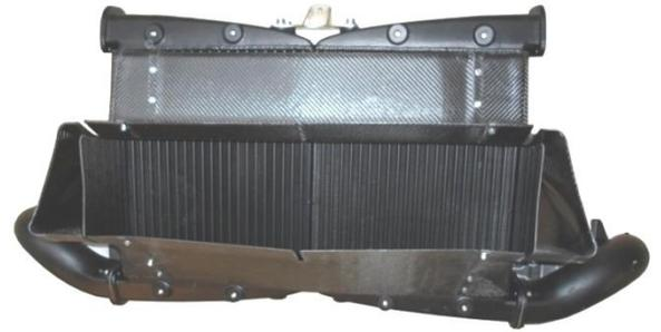
**4. Montage Ladeluftkühler / mounting Intercooler**
